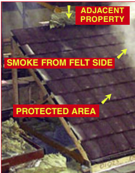
DURING THE FIRE TEST
