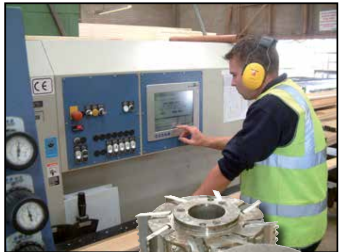
The moulding machine at Quarry Lane being set up for a production run. Inset shows examples of typical cutting heads.
