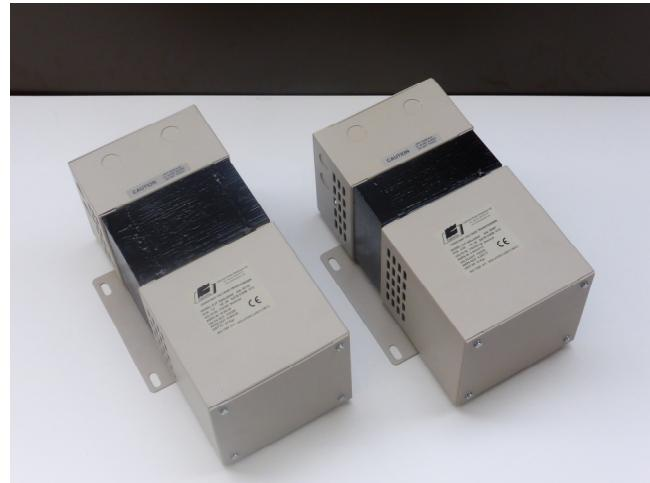
The main feature of all Constant Voltage Transformers (CVT) models is the ferro-resonant principle of operation, proven to be the effective way to cure the problems of mains interference and irregular voltage.
