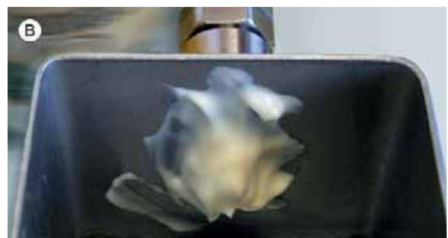
(A) The LMT sensor monitors the level of mayonnaise using the high-frequency capacitance spectrum profiling technology. (B) Despite deposits on the sensor the empty tank is detected reliably.
