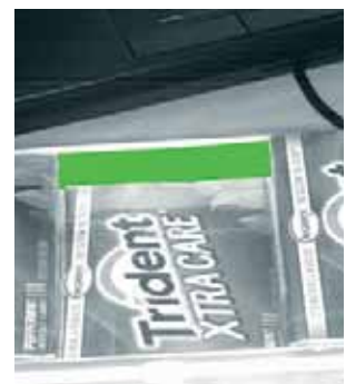
(B) The pixel counter detects if one layer is missing by means of the visible area at the inside of the cardboard box.
