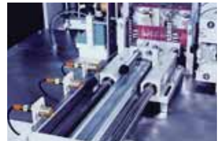
Typical application: Positioning sensing in automation technology; inductive sensors operate reliably and without wear.
