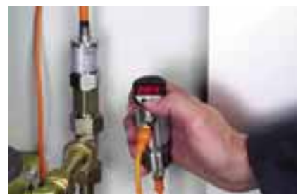
Separate display / programming unit PP2001.
