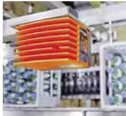
Completeness check in the bottling process with efector pmd3d.
