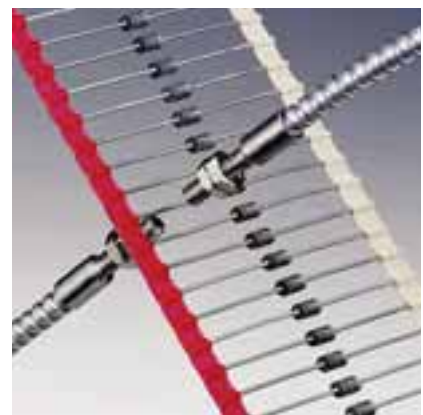
Minute objects up to 0.5 mm are detected safely.
