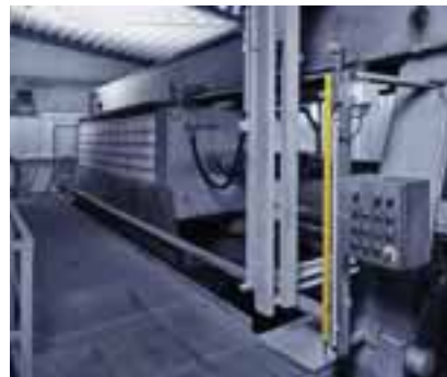
Area monitoring by means of safety light grids.
