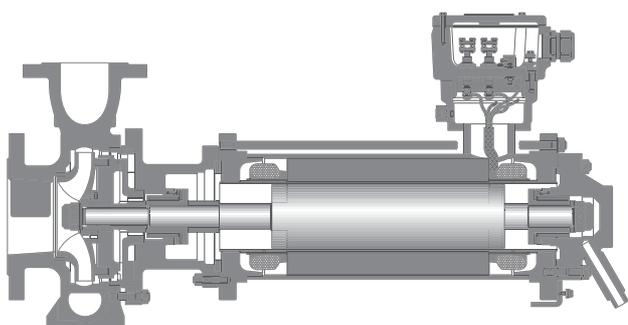
Single-stage canned motor pumps
