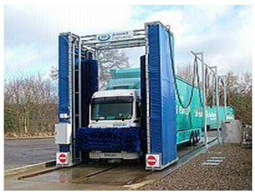
The three brush wash machine is the preference for the cleaning of conventional road going commercial vehicles. This equipment is designed to wash vehicles quickly and effectively ranging from medium sized vans to large articulated units and trailers.
