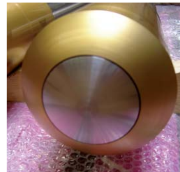
Piston head with tungsten carbide coating
