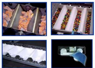
Gough buckets are designed to handle the tough AND sanitary applications. With several bucket sizes available, product throughputs can be handled gently without spillage. A variety of bucket materials allows for the right bucket for the right application.
