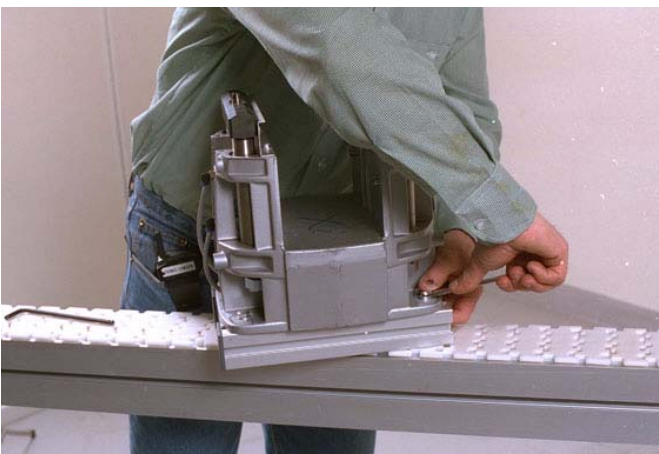
7 Tighten all screws.
