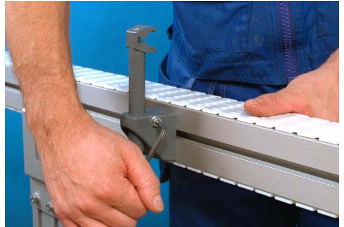
2 Attach a guide rail clamp to the bracket. Tighten the screw.
