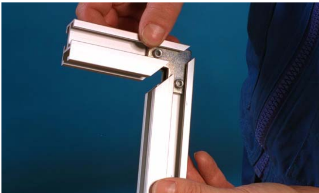
b) L bracket Type 2: Use a XMRW 20 corner fitting to connect two beam pieces that have been cut in a 45° angle.
