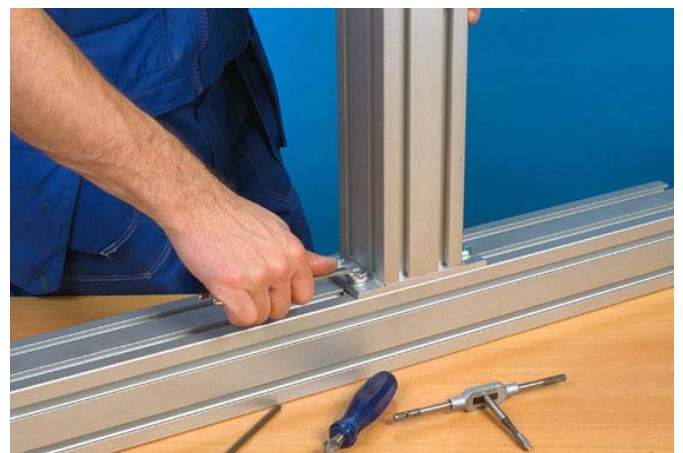
4 Screw the mounting plate onto the side of the transverse beam using hex head screws M6S 8x16.
