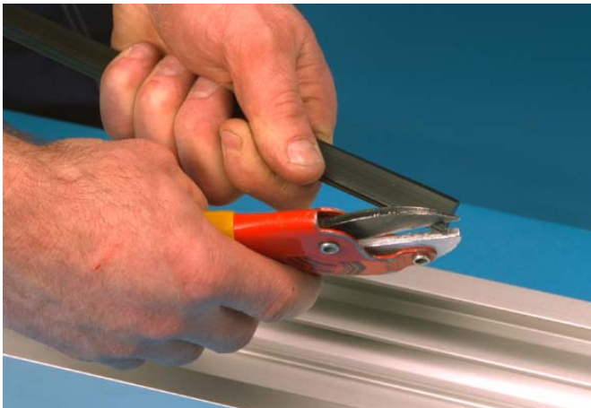
1 Cut the slide rail in a 45° angle.
