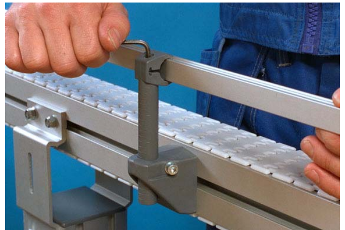
3 Attach the guide rail to the clamp. Tighten the screw.
