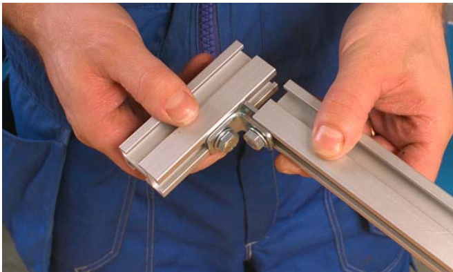
1 a) L bracket Type 1: Use a XMRY 20 inner fitting to connect two beam pieces. Tighten screws.
