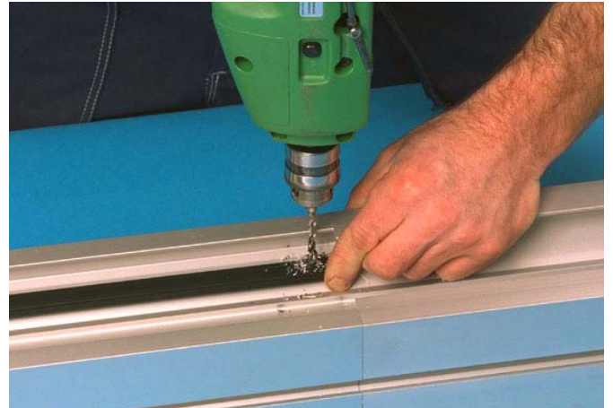
3 Drill holes for plastic XWAG 5 screws.
