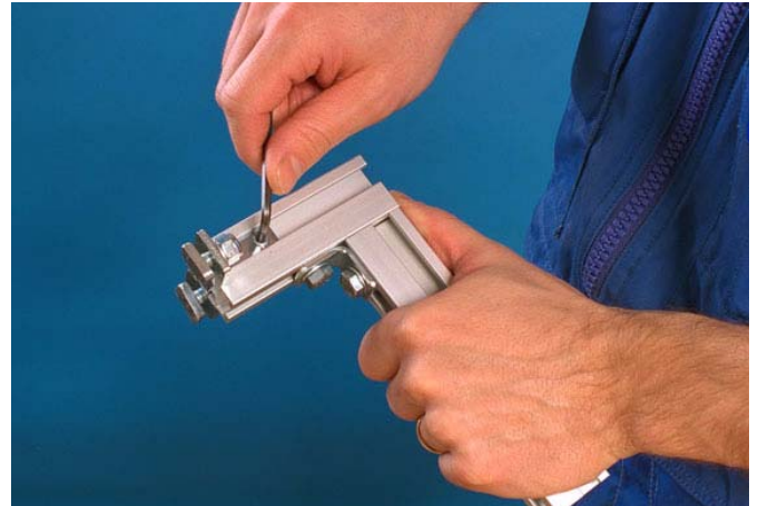
2 Attach two XMRX 20 inner fittings to the end of the L-bracket.
