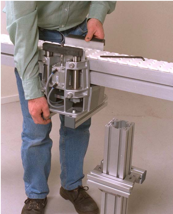
10 Lift up the locating station and fit the guide pins into the T-slot on one side of the conveyor beam.
