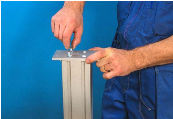
1 Attach a mounting plate to the beam end using MF6S 8x30 hex socket head screws and washers.
