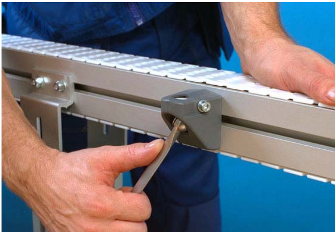
1 Fasten a guide rail bracket support to the conveyor beam using T-bolt, nut and washer.
