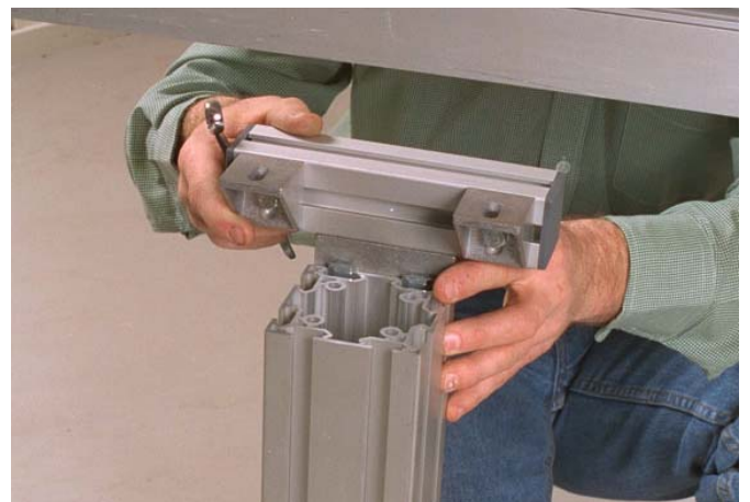
9 Insert square nuts in the vertical beam T-slots. Use angle brackets to mount short pieces of XCBM 44 beam on the vertical beam.
