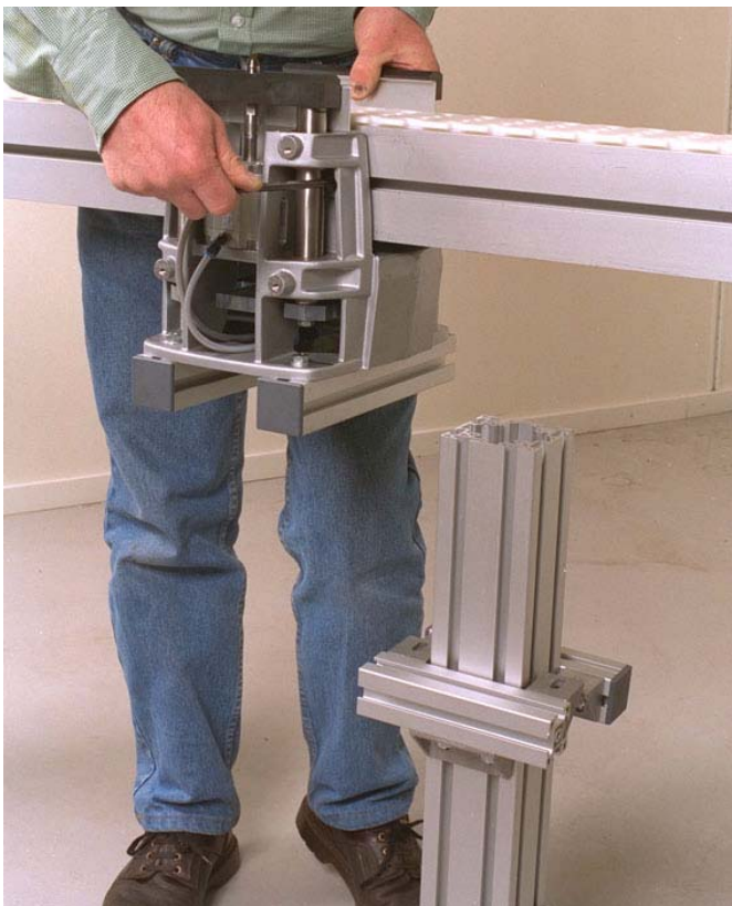
11 Tighten the two remaining guide pins.
