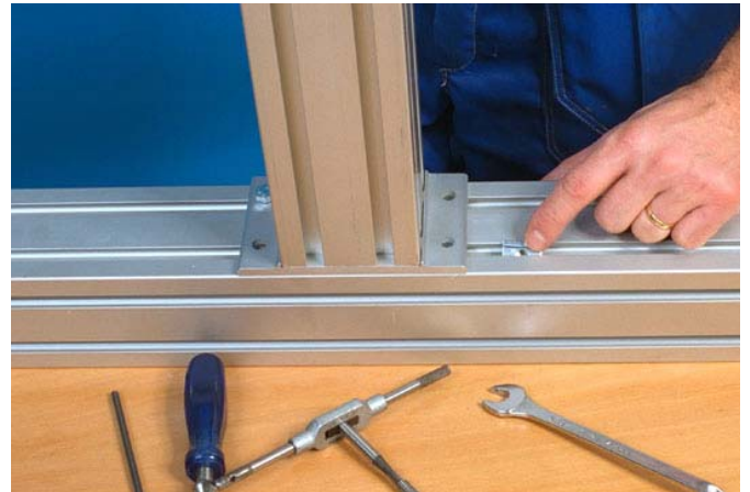
3 Insert slot nuts into the T-slots of the transverse beam.
