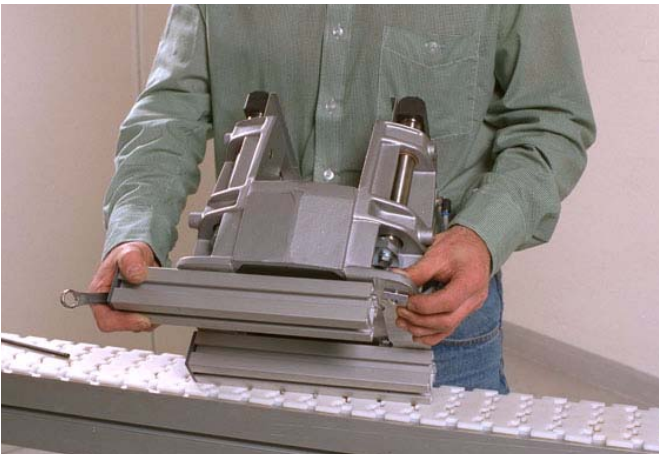
6 Remove the cover from the locating station. Mount a pair of XCBM 44 beams ( \approx 270 mm long) underneath the locating station, using M6S 8x20 screws, washers and XCAN 8 slot nuts.
