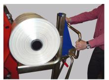
The trolley can be used to load master rolls & unload large rewound rolls.
