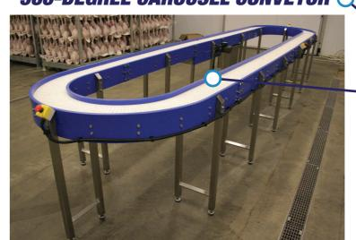
Transporting trays of Turkeys to a number of operator stations for preparation and packing.
