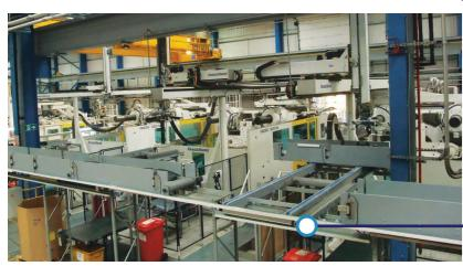
Transporting automotive components from a moulding machine robot to a packing line.
