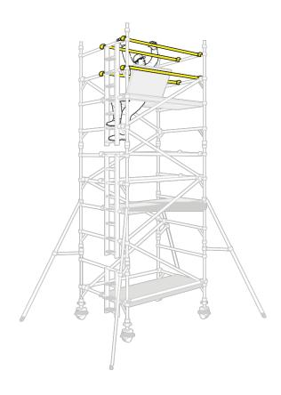
Continue until the required height is reached. Re-position the fixed deck to the required platform height and fit a trapdoor deck alongside it as shown in <a href="stage">stage</a> 7. Fit a single diagonal at the top of the tower as shown in <a href="stage">stage</a> 7. Fit the final guardrails as shown in <a href="stage">stage</a> 7.
