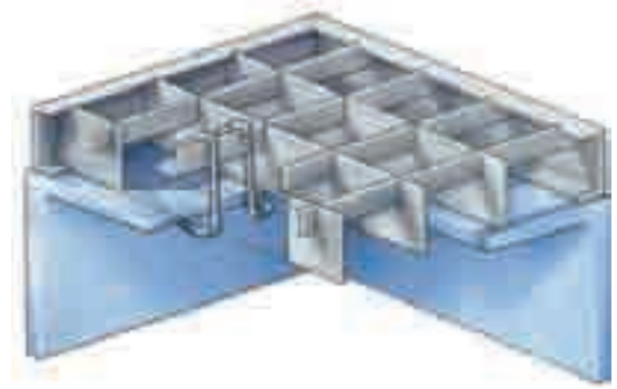
Attachment spring for easy assembly and dismantling of gratings on steel structures. It is designed as a spatial spring and replaces conventional standard and double clamps.
