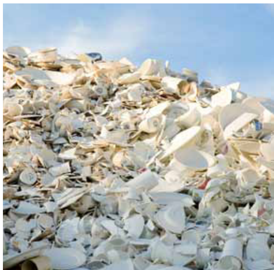
All ceramic tiles manufactured by Johnson Tiles at our Stoke-on-Trent factory now contain up to 28% recycled ceramic material from our own ceramic waste recycling scheme.
