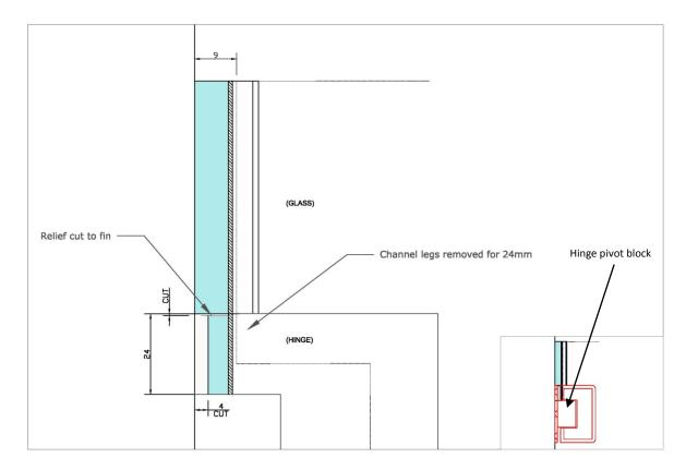
Follow the same process for the bottom hinge, making sure the (S05) seal is the right way round when cutting (fin on the inside).
