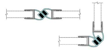
Seal wall attachment needs to be drilled and screwed to wall then seal can slide on.
