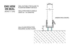
The hinge side has a flexible fin see below, jamb side to a wall has central fin.
