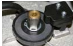
Mechanical twin-disc clutch (only for SATURN OIL)
