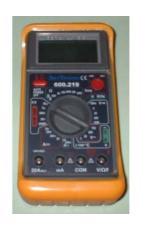
A highly featured digital multitester for professional use. Offers 30 ranges and 8 functions including temperature, capacitance, diode, continuity and hFE measurement. Large 3.5 digit LCD display with automatic polarity indicator. Supplied with shrouded test leads, K type temperature probe and shock proof rubber holster.
