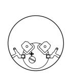
This is available as a rear mounted factory fitted option. The unit contains a Ø 6mm 'festoon' style lamp available in 6V, 12V or 24V. Please contact the sales office for more
