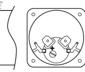
This is available as a rear mounted factory fitted option. The unit contains a  $\emptyset$  6mm 'festoon' style lamp available in 6V, 12V or 24V. Please contact the sales office for more
