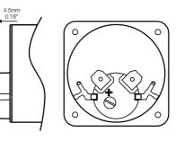
This is available as a rear mounted factory fitted option. The unit contains a  $\emptyset$  6mm 'festoon' style lamp available in 6V, 12V or 24V. Please contact the sales office for more
