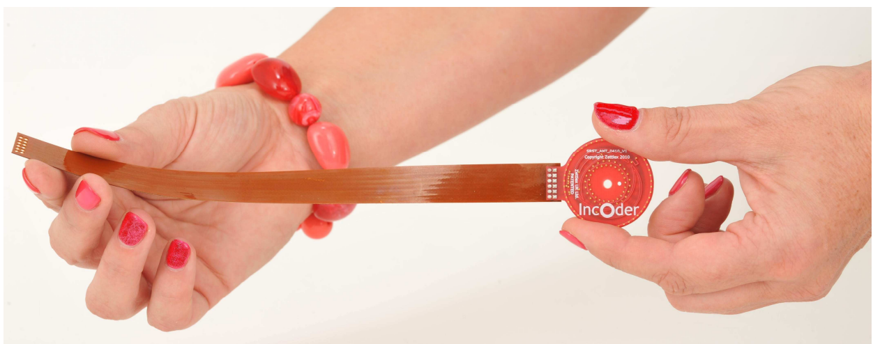
Fig. 5. – Next generation inductive sensors are as compact as pots and mimic their analogue output
