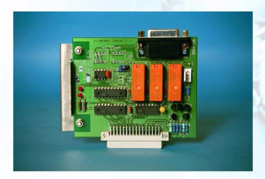
As standard, the complete range of Time & Frequency Solutions' timing products include self-test and diagnosis capability. This feature is known as BITE (Built in Test Equipment).
