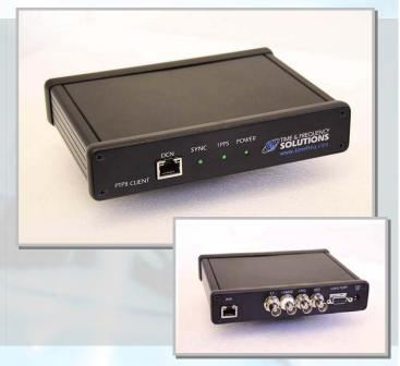
The PTP8 Slave Network Time Client converts the IEEE1588v2 protocol supplied across a packet network to traditional E1/T1, 1PPS, 10MHz, IRIG B, Serial TOD and customer requested timing signals.
