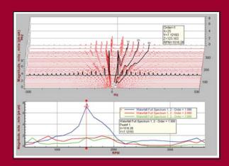
measurement suite handles simultaneous asynchronous and synchronous sampling and provides both vector and waveform samples while also recording raw data to disk for optional post processing. Order detection is based on user selectable tracking filters which may be set up as fixed or proportional bandwidth permitting users to optimize accuracy for varying slew rates. In addition to 1x and 2x, up to 6 other tracked orders are available per measurement channel.
