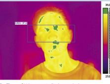
The ThermaCAM automatically detects the hottest temperature within an area, set by the operator. A color alarm makes it easy to decide whether a person needs further examination or not.
