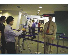
Setting up a ThermaCAM with Automatic Temperature Compensator (ATC) for viral disease detection.
