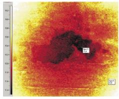
Thermal images show a reccurent critical situation detected on the Façade, concerning fractures and water stagnation in stucco works (darker area)
