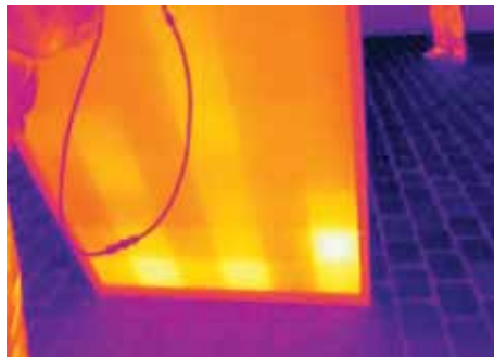
These images taken from the back of the same solar panel show much less reflection than the front, making the temperature measurements much more accurate.
