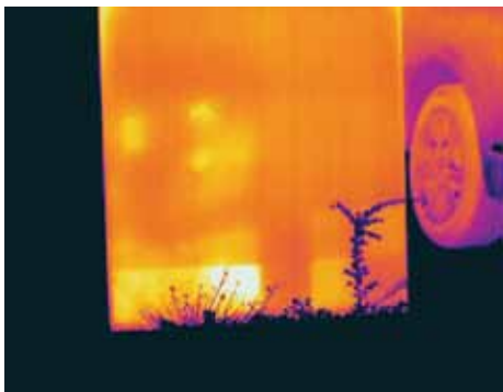
These hot spots seem to indicate inefficient solar cells, but closer inspection shows that several of the hot spots are caused by the reflected warmth of people standing in front of the panel.
