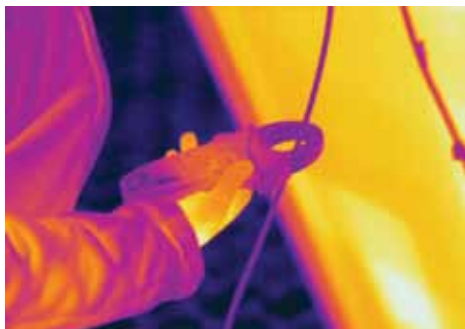
The amount of electricity the panel produces can quite easily be measured with the clamp meter. The measurement data are combined with the thermal image with the help of FLIR MeterLink technology.
