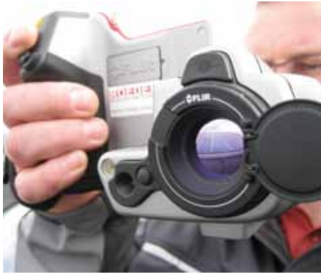
The FLIR T335 thermal imaging camera is available with several different interchangeable lenses.
