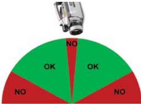
Viewing angle recommended (green) and to be avoided (red) during thermographic inspections.
