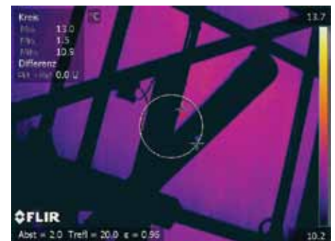
The hot spots on this thermal image taken from the front of the solar panel might seem to indicate that a multitude of cells are working inefficiently.
