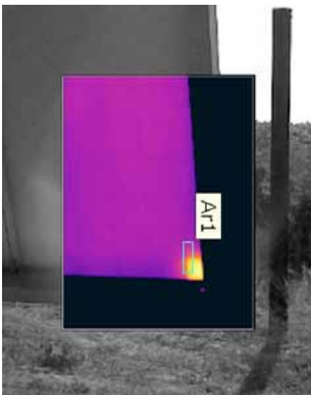
This Picture in Picture image shows a hot cell due to a shadow from the nearby alarm system.
