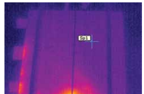
This thermal image shows that this cell has flaws in the edge isolation, which causes local shunts.
