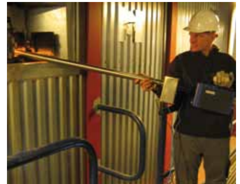
Temperature measurement through a port
