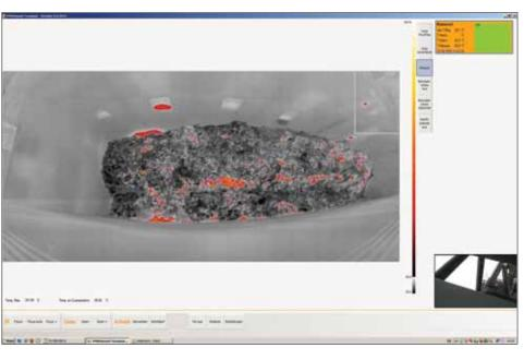
The PYROsmart system clearly shows the areas that are susceptible to spontaneous self combustion. The fire monitor will cool these areas down.
