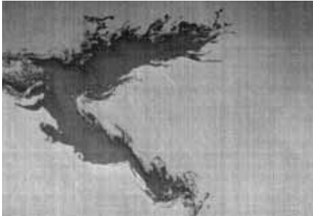
A visible image and a thermal image of Doba/Chad crude oil, at a low camera angle, a glassy calm sea state, in full daylight.
