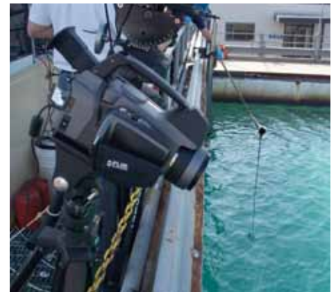
These FLIR thermal imaging cameras are pointed at oil spills in the OHMSETT tank at different angles.
