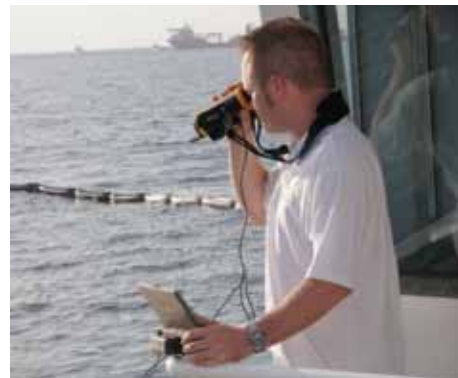
An oil recovery operator uses a FLIR HM-Series handheld thermal imaging camera to direct the positioning of oil recovery booms.
