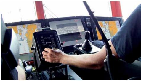
In the Stormbull's cabin two multifunction displays and one dedicated display give all three crewmembers continual access to the Voyager's thermal images. The ergonomic Joystick Control Unit (JCU) is mounted in the middle.
