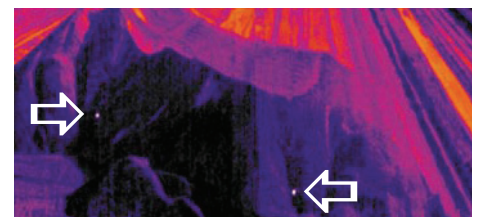
The overlay of a coal pile with 2 hot spots as possible combustion points.
