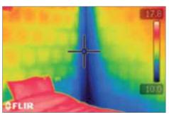
The temperature difference between the cold area in the corner and the rest of the wall is over 5°C.
