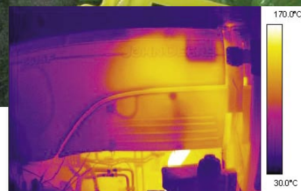
Checking hood surface temperature distribution
