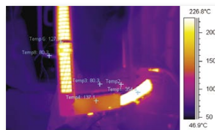
Checking hood surface temperature distribution
