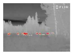
The unique InstAlert feature colors the hottest parts in the thermal image red, making it extremely easy to spot animals in the thermal image.
