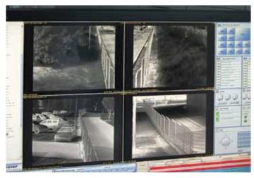
Visual analysis software is much more effective when connected to thermal imaging cameras. "A trespasser shows up very distinctly due to the thermal contrast", explains Krüger.
