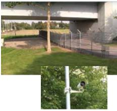
These thermal imaging cameras from FLIR monitor one of the flood-threatened areas. They need no lighting to be effective and due to their long range capacity they can cover the entire area from a safe distance.
