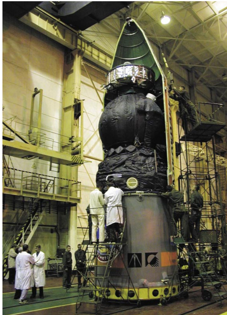
Foton-12 being installed in the fairing system of the Soyuz rocket. Through observations made with the aid of the FLIR Systems' camera, scientists discovered a phenomenon in the behaviour of fluids in weightlessness conditions that adversely influences crystal growth.
