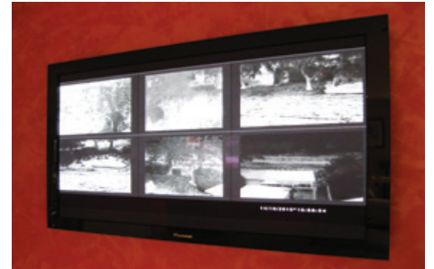
The thermal images of the six FLIR SR-313 thermal imaging cameras can be shown on any of the screens inside the house.
