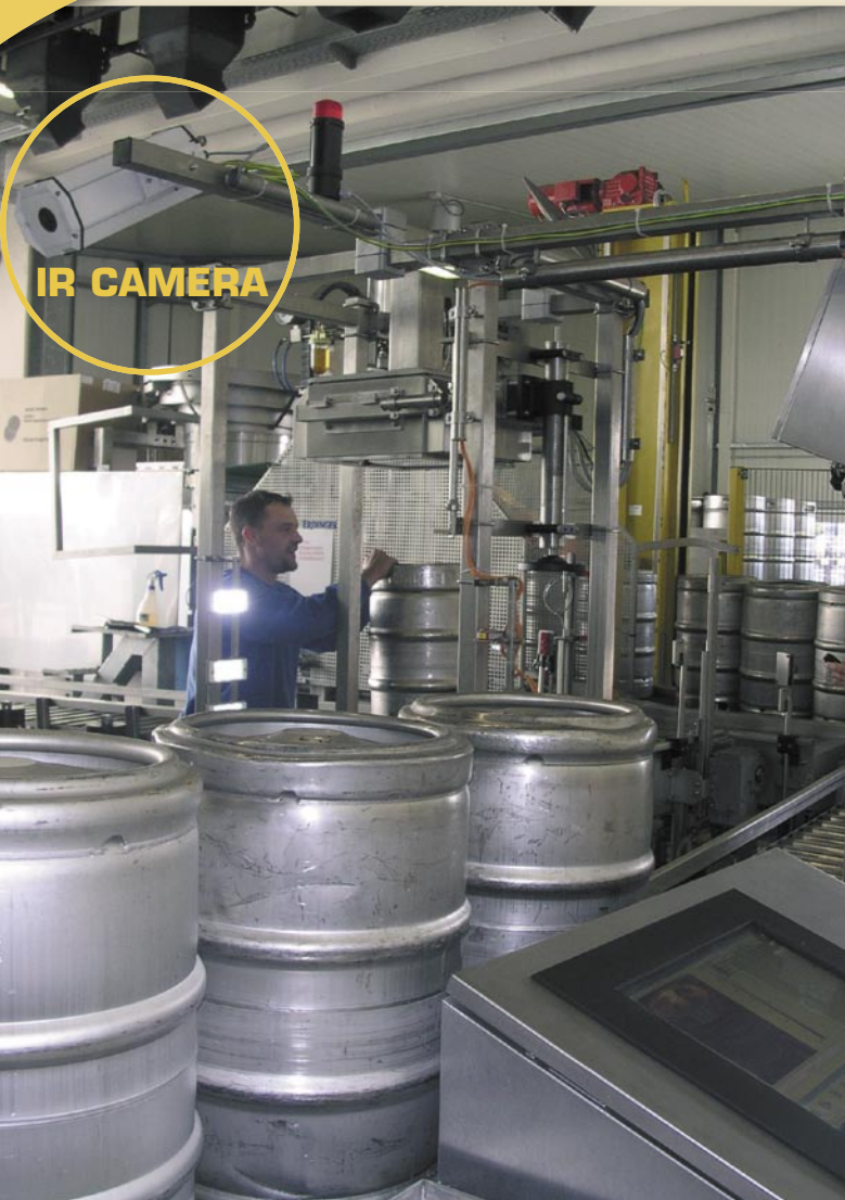
The infrared camera (top left in the image), checks each passing keg.
