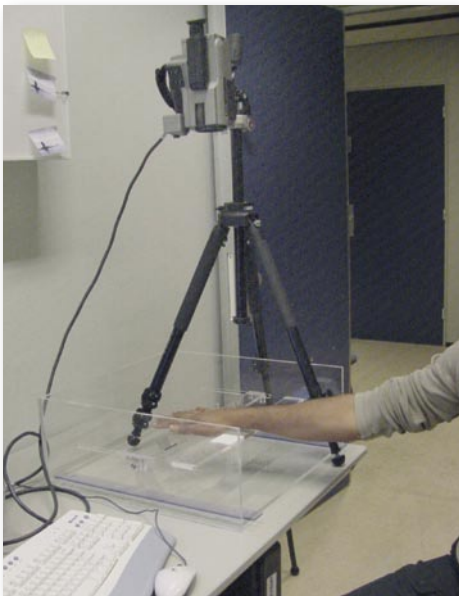
Measuring the temperature of the hand of a CRPS patient with a ThermoCAM.
