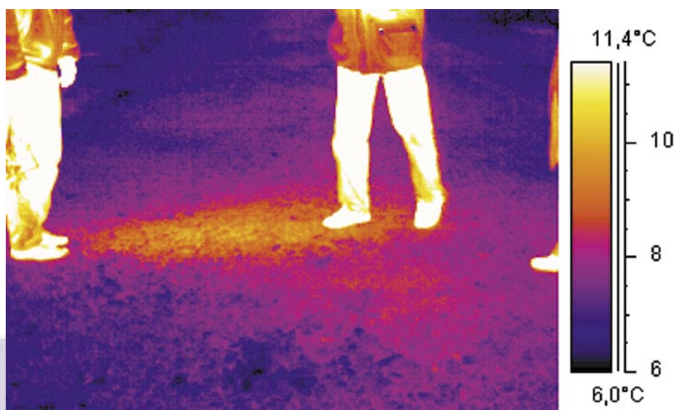
Thermal images produced by the FLIR ThermoCAM provide detailed information that is invaluable to accurately locate leaks or damages in district heating networks.
