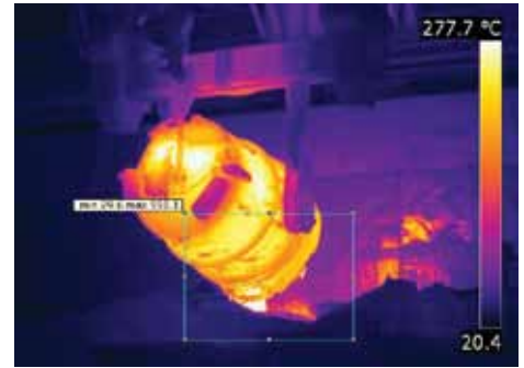
The refractory on this ladle shows signs of wear and if it degenerates further needs to be replaced. Thermal imaging cameras are the only practical tool available for refractory inspections.
