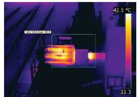
This electromotor is overheated and needs to be inspected and repaired before a failure occurs.
