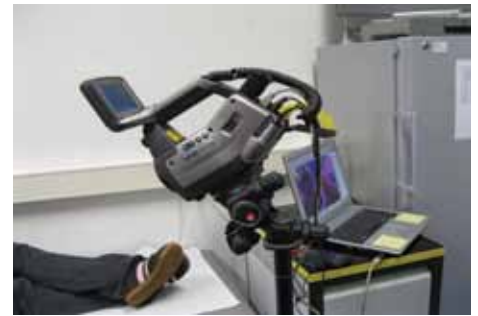
The thermal imaging camera from FLIR is plugged into the laptop through a FireWire connection.
