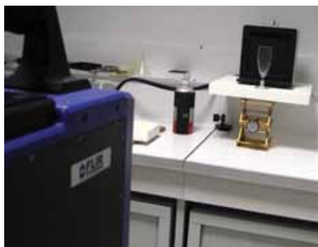
The SC7000 operates at a bandwidth of 3 to 5 μm, the external filter narrows it down to exactly 4.245 μm.
