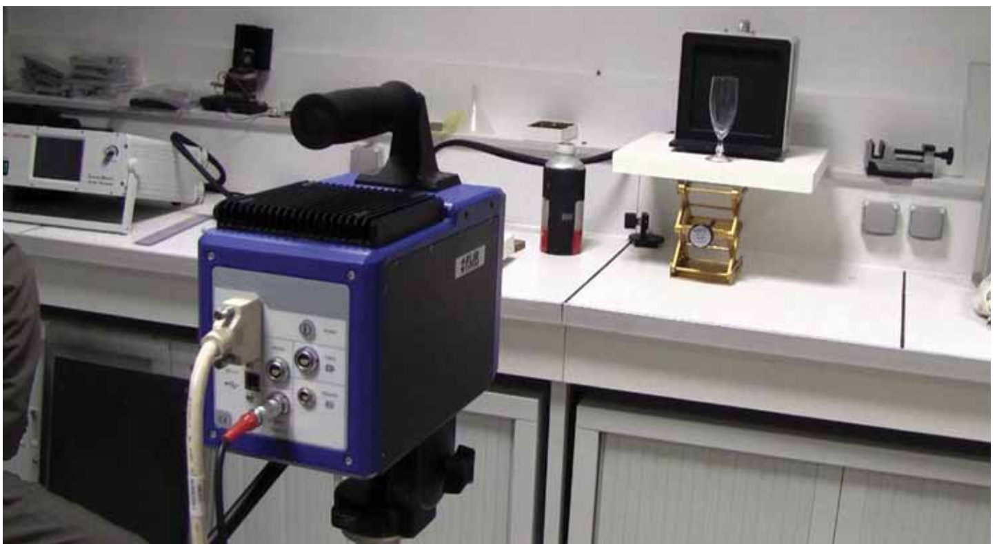
The FLIR SC7000 thermal imaging camera is pointed at a champagne flute standing before a calibrated blackbody.
