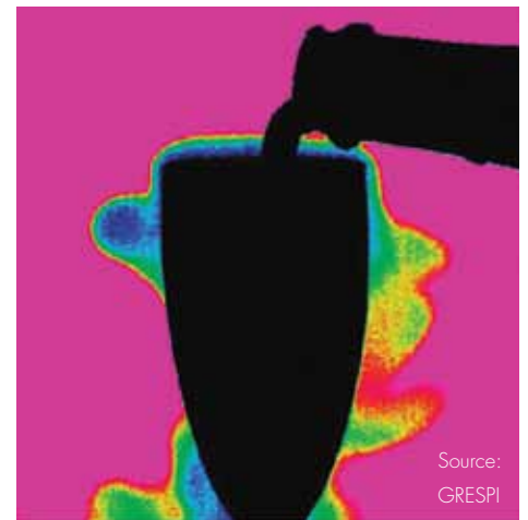
Researchers used a FLIR SC7000 series thermal imaging camera to visualize CO 2 as it escapes during the pouring of a glass of champagne.
