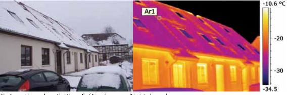
This thermal image shows that the roofs of these houses aren't isolated properly.
