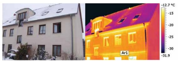
In this example it is clear that the rightmost skylight is leaking warmth at the frame and there are several locations where the roof insulation isn't very effective.
