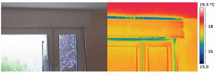
If you look at it, this window seems pretty airtight, but during a Blower Door test with a FLIR thermal imaging camera the draft clearly shows on the thermal image. Tests with the anemometer showed air flow of 6.44 m/s, which is extremely high, considering that everything above 2 m/s is considered to be a strong air flow.
