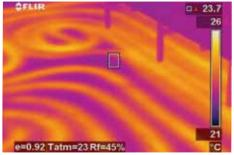
The FLIR B660 is also an excellent tool to test the effectiveness of under floor heating.
