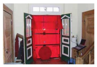
A Blower Door test consists of a ventilator that's installed in a doorway, sucking air out, which causes the outside air to rush into the building through available cracks and crevices.
