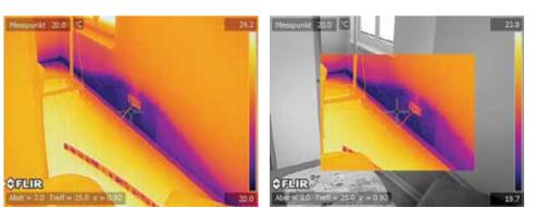
This case of water damage clearly shows the advantage of the Picture-in-picture feature, since the client can quite easily see where this thermal image is located, while this would be more difficult with only the thermal image.
