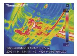
Another practical example is the study of the heat transfer of catalysators. Located at the back, underneath the car, it disperses an enormous amount of heat. With the help of infrared thermography the heat dissipation is being studied, to avoid that, for example the trunk of the car, overheats.
