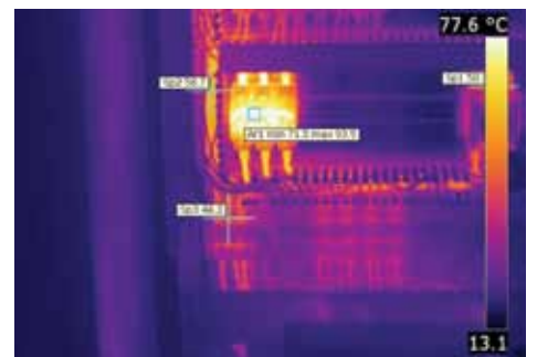
The fuses that show up in the thermal image are overloaded and need to be replaced.
