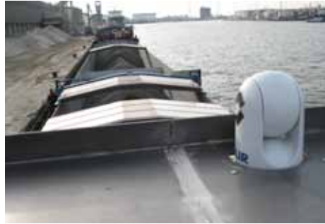
From this vantage point the FLIR M-Series thermal imaging camera can make the most of its wide field of view and excellent range performance.
