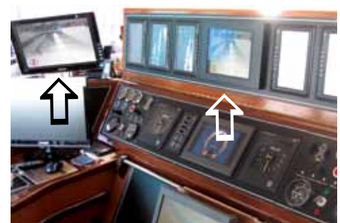
The thermal imaging footage from the FLIR M-Series is continually displayed on one dedicated screen and one multi-functional screen on the bridge of 'El Niño'.
