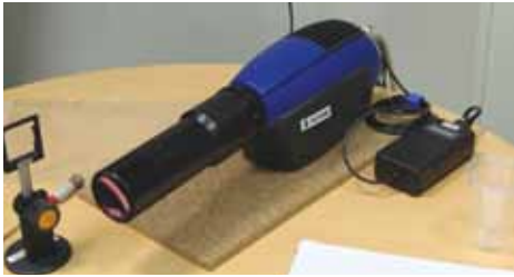
The SC5000 thermal camera is available with a wide variety of different lenses.
